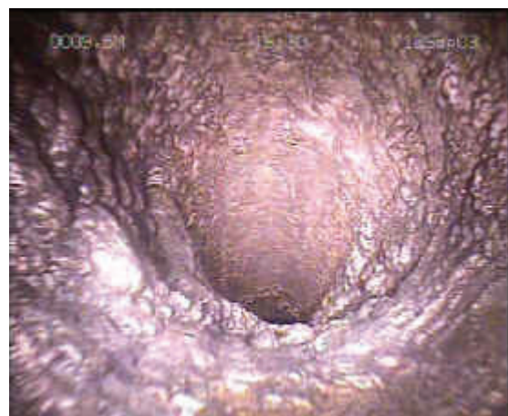
Figure 3 – Scale at Riser Top (2003)
