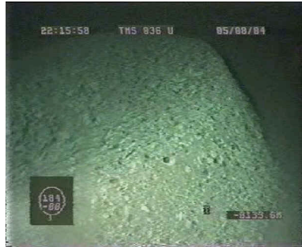
Figure 9 – Scale Mound from Riser Cleaning
